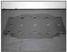
Locate base and place white side down. The pallet base should be positioned so the length is in front of you and the width is on the side.
