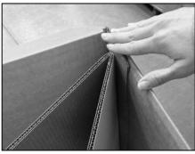
Place stabilizing inserts into box with longest side fold in the corner of the box with the glued seam.
