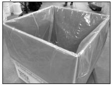
Add liner to box and fold over flaps of the box. Open liner into all four corners of the box to avoid bunching.
